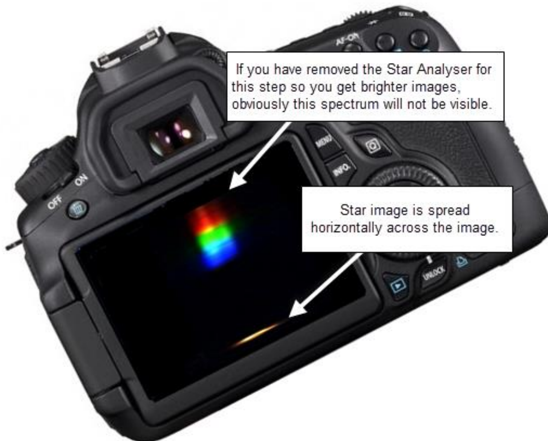
Figure 3: When the camera is properly flipped, the star image will smear horizontally across the image in long duration exposures.
